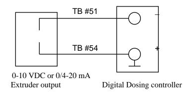
Figure 6. Analog Extruder Input Connection Diagram – Extrusion - Proportional
